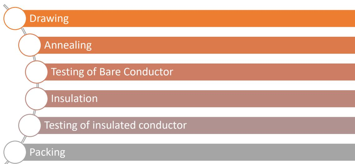
1. **Drawing:** In this process the aluminium / copper rods are drawn into wire/ strips (flat wire) through rod breakdown machine (for round wire) and conform machine (for strips). Wire/ strips are drawn in different sizes depending on the customer demand. We produce wire in the range of 0.19 mm to 4.00 mm and strips in the range of 5 mm sq. to 300 mm sq. We have sophisticated fully automatic machines which are capable of drawing wire / strips in different sizes.
